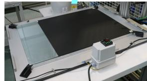
A build platform uses several thermostat-controlled heaters below a large aluminium block to keep a glass bed heated during printing.
