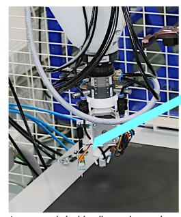
An automatic bed leveling probe was integrated into the extruder tool. The probe allows for automatic leveling of the build platform. A servo controls the deployment and stowing of a touch probe. This ensures that the probe stays out of the way during the printing process, which aids in freeform printing.
